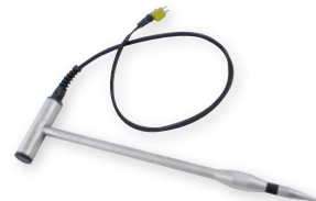
GSF 50TF (110 cm) Art. no. 601312 GSF 50TFK (43 cm) Art. no. 601313 Material moisture insertion probe, with temperature sensor, for measurement up to a depth of 40 cm or 107 cm, incl. 1 m connection cable. Suitable for: wood chips, wood wool, straw, hay, grain, saw dust, etc.
