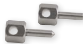
GST 15B* Art. no. 601281 Steel pins 2 steel nails with bore hole, 15 mm long, Ø 3.8 mm (for direct connection of measuring cable GMK 38)
