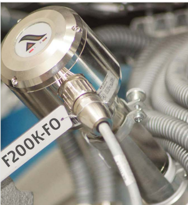
F200K-FO Fibre Optic implementation
